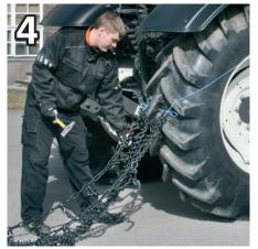
Drive forward one circuit, keep the chain narrow.
