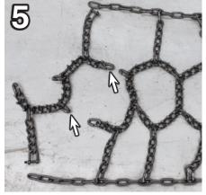
If the chains have a removable extension, remove it from slanted gap links if needed.
