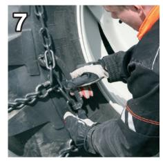
Fasten the chain with the fasteners, inside first and then outside.
