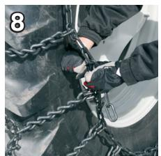
A good rule is that your hand should fit between the tire and the chain. Do not tension too tight. Hammer the plugs of the couplers.
