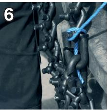
When the chain ends meet, connect the links slanted gap upwards. Remove the rope.
