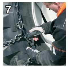
Fasten the chain with the fasteners, inside first and then outside.
