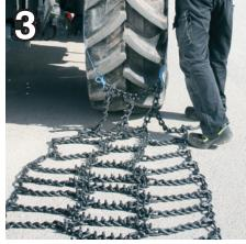
Put the rope on the top of the tire.
