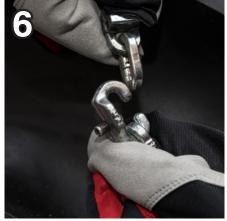
When the chain ends meet, connect the links with plug couplers - center first. Remove the rope.
