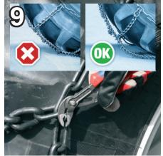
Check the tightness of the shackles and the chain after a short test drive.
