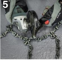
In most cases the chain must be cut to fit perfectly. Always make the cut from a studded link. Don't cut the chain too short.
