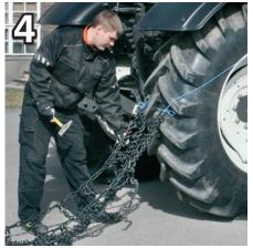
Drive forward one circuit, keep the chain narrow.
