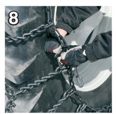
A good rule is that your hand should fit between the tire and the chain. Do not tension too tight.
