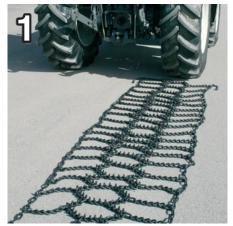
Put the chains behind the tire with the fasteners against the tractor and the studs facing up.
