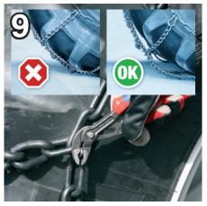
Check the tightness of the shackles and the chain after a short test drive.
