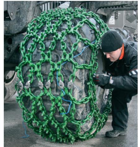
7. Tighten the tension chain with shackles. Note, tension chain is not a standard option for all chain models.
