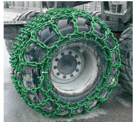
10. In daily service, tighten only the tension chain. Thus chain mesh is widening and the chain shortening. Shorten the chain when tension chain reserve is used.
