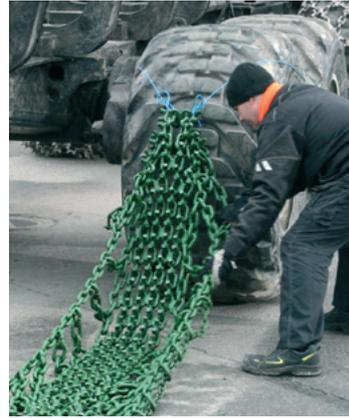
3. Drive forward and keep the chain pattern as narrow as possible. Don't spread the chain. Use hammer if the chain is too sticky.
