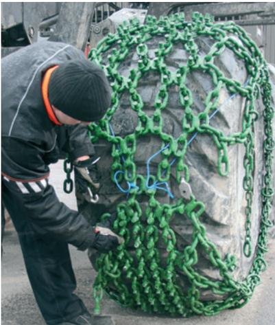
5. Fasten pin couplers and remove the rope.
