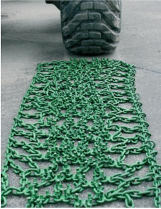
1. Put the chains behind the tyre, studs facing up. If the chain includes tension chain, it should be outside.
