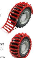
**TRACK TENSION:** The removal of one full track plate may be required to obtain the correct tension. This may be dependent upon whether the track is fitted to new or worn tyre.
