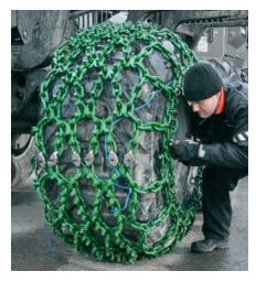
7. Tighten the tension chain with shackles. Note, tension chain is not a standard option for all chain models.
