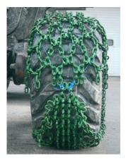
4. Stop the machine when chain ends are on the same level.
