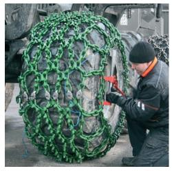
6. Fasten side chain with shackles, both sides exactly to the same length. Tighten first the inside chain and then the outside. Don't tighten the shackles too tight at this point.
