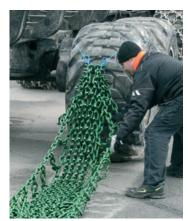
3. Drive forward and keep the chain pattern as narrow as possible. Don't spread the chain. Use hammer if the chain is too sticky.
