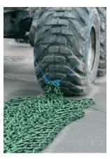
2. Fasten the rope middle of the chain. Put the rope on the top of the tyre.
