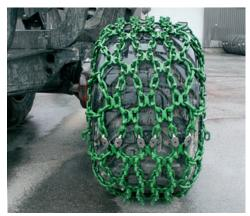
9. Drive 20-30 meters and tighten tension chain if needed. Tighten all shackles. Check tightness of the chain in daily service.
