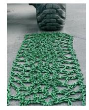
1. Put the chains behind the tyre, studs facing up. If the chain includes tension chain, it should be outside.
