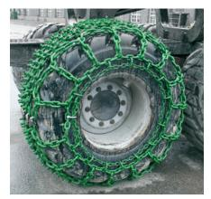
10. In daily service, tighten only the tension chain. Thus chain mesh is widening and the chain shortening. Shorten the chain when tension chain reserve is used.
